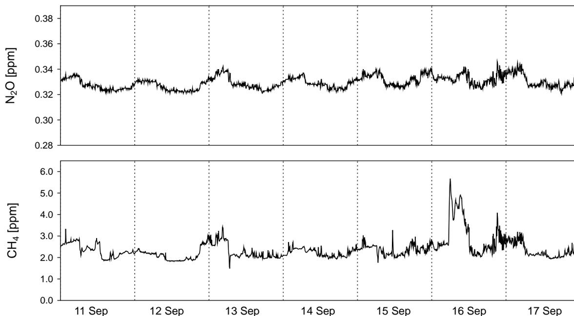
Fig. 6. N<sub>2</sub>O and CH<sub>4</sub> concentration curves for September 2001 measured with the FTIR and multi-pass White cell (~ 23 m). Dotted lines correspond to midnight hours.
