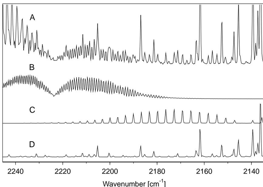
Fig. 3. FTIR spectral window showing: **A** one sample spectrum and **B** N<sub>2</sub>O, **C** CO and **D** H<sub>2</sub>O reference spectra computed with E-Trans.
